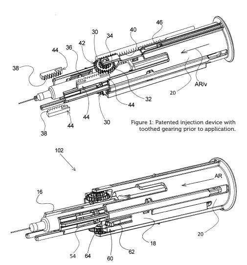
Figure 2: Patented injection device with toothed gearing during application.
